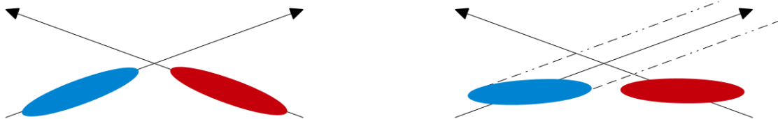
Figure 4-1: Bunches colliding with a crossing angle without (left) and with (right) the crab crossing
