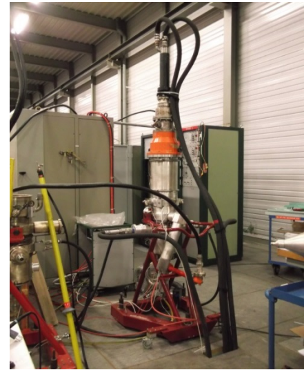
Figure 4-23: Cryomodule and RF system layout in the LSS44 cavern (left) and a 400 MHz Tetrode amplifier under test (right).
