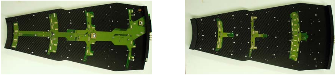
Figure 3.32: The different ICBs on the two sides of a front petal: ICB_2 and ICB_46 on side B, and ICB_1, ICB_3 and ICB_57 on side A (from left to right). On ICB_46, the two CCUMs are plugged.
