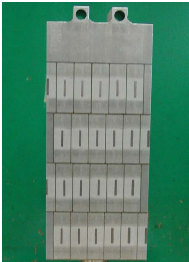
Figure 2.4: Cross section of the cold mass with the details of the 4-layer winding with reinforced conductor.
