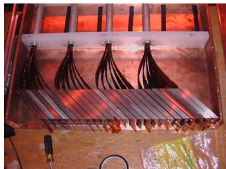
Figure 6.5: Photograph of the ZDC HAD section.
