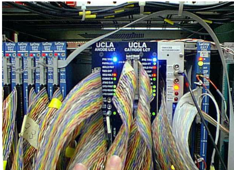
Fig. 11.13: CSC trigger prototypes for the 1998 test beam at H2. From the middle to the right of the picture are shown: ALCT, CLCT, and TMB modules. On the left are shown anode readout TDCs.
