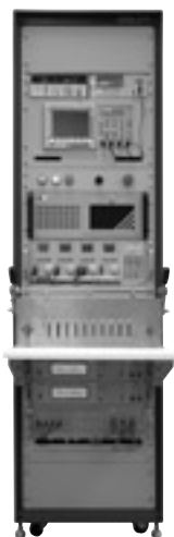
DC to DC Converter ATS
