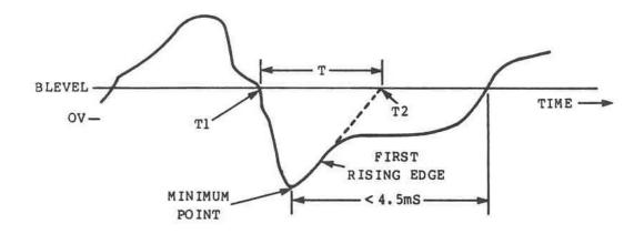
Figure 1. Typical Waveform. The level of the waveform in the region between the first rising edge and the second one is unknown and variable. The time from the minimum point to the next baseline crossing is less than 4.5mS in all test runs.
