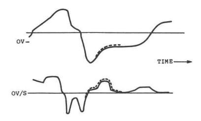
Figure 2. Measured Waveform (top), approximate differential waveform (bottom), and cursor set over first rising edge (dashed line).
