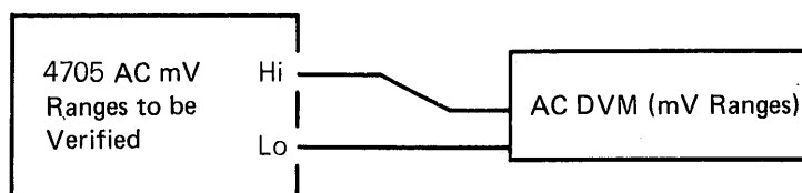
Verification of 4700 LF Millivolt Ranges
