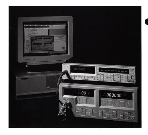
The hardware contains no physically adjustable circuit elements; calibration corrections are stored in two non-volatile memories designated "Baseline" and "Certified". Baseline calibration constants are determined at manufacture and remain stored within the instrument for life to enable its performance to be readily monitored. "Certified" calibration constants are stored during comparison to standards for the specific calibration of the subject calibrators.
