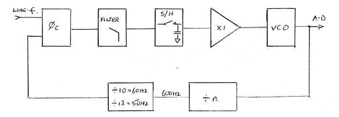
**DIGITAL FILTERING:** Improvement on the basic 60 to 70dB SMRR obtained from an integration over one power line cycle (PLC) can be achieved by integrating over a number of PLCs, thereby averaging out the effects of line-f "jitter".
