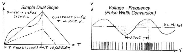
In these techniques the areas under the curve of the AC component cancel out, resulting in the measurement of the MEAN or DC level only.
