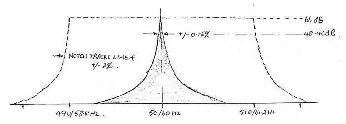
The effectiveness of this rejection Notch is very much qualified by the ability of the DMM's line locking circuit to track (hold lock on) small shifts in line frequency. Utility authorities generally specify frequency stabilities in the order of +/- 1%.
