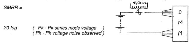
The most significant source of AC interference is the frequency of the utility supply, 50Hz in Europe and 60Hz in the USA and much of the Far East.
