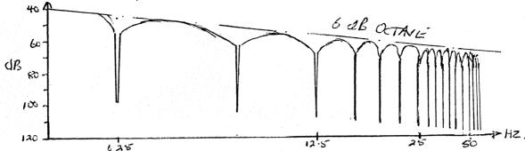
AVERAGING: Another technique employed to improve the SMRR, and to give a quieter display, is post A-D averaging, where the user can choose to average over a number of readings. The Selfcal DMMs provide for both "Block" and "Rolling" average.
