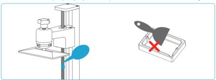
3.Be careful when you remove the build platform in case you may smash the 2K Photocuring screen. 4.If you don't use the printer in the next 48 hours remember to put the left resin in the tank back to its bottle and seal it. And if there are any residues please use a filter to filter them out.
