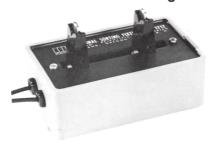
This fixture holds components for test while providing four-terminal connection. Its holding clips can rotate 90 degrees to accommodate axial and radial-leaded components. They can also be set from 116cm (5/8 in.) to 8cm (3½ in.) apart. This allows use of this fixture with many component sizes and configurations.
