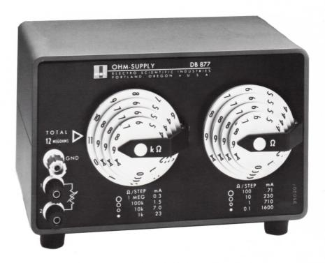
Featured is the ESI-patented Dekadial® coaxial dial arrangement which provides up to 120 million divisions of resolution. It allows first, coarse approximation and then progressively finer steps to arrive at an exact resistance value. The dials turn independently through 360 degrees of rotation. A special detent design facilitates dial location.
