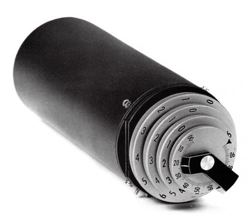
These Dekapot potentiometers are precision decade resistive voltage dividers featuring the accuracy, high resolution, and constant input impedance of the Kelvin-Varley circuit. They provide known voltage and current ratios for meter calibration, linearity checking, ratio measuring, synchro testing, computer standardization, and many other DC and audio frequency applications.
