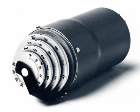
The Dekatran® decade ratio transformers are inductive voltage dividers for use at audio frequencies. They feature high input impedance, low output impedance and low phase shift and are ideal for use as working standards in test setups and calibration laboratories. Applications include voltage and current division, turns-ratio measurement, divider calibration and impedance comparison.
