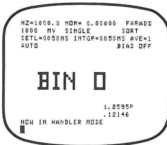
Figure 3-2. -8 CODE and 26 CODE Display Format
