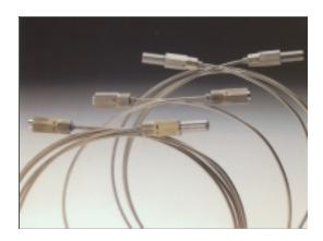
The Fenwal sensing element consists of a coaxial assembly, with a center conductor. Surrounding the center conductor is a eutectic salt compound embedded in a porous ceramic material, which at normal ambient
