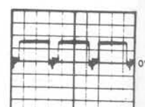
EACH DIV. = 0.5V, 20μs BASE of Q2
