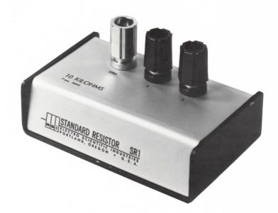
Terminals appear on the top of each unit. They are also brought out the bottom of the case on removable banana plugs. This allows plugging two or more units together in either series or parallel for a wide variety of resistance values. Four-terminal resistance measurements are easily made by using the banana plugs on the bottom of the case as two of the terminals.
