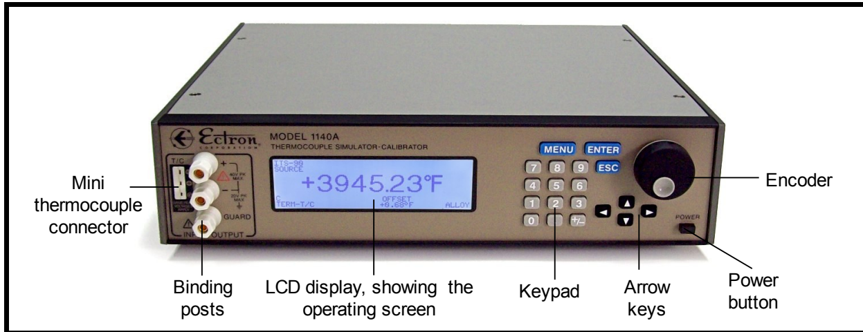
Figure 4-1: Front View of the Model 1140A
