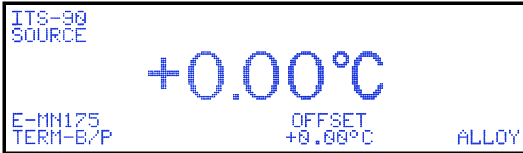
Figure 11-5: Operating Screen for Thermocouple Alloy Tests
