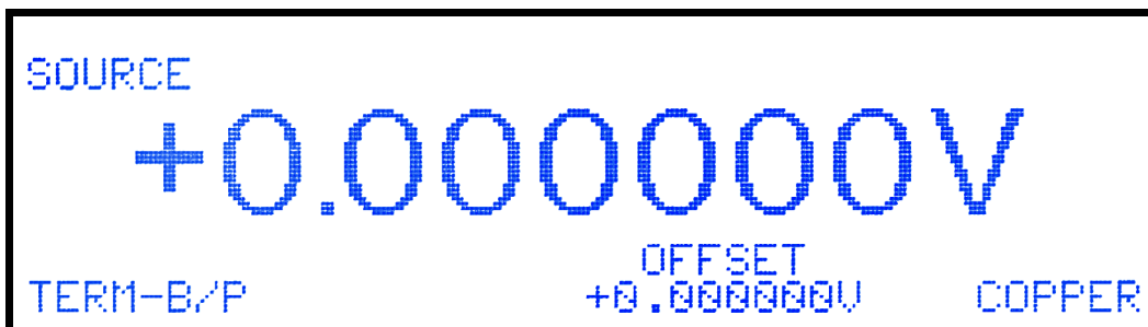
Figure 11-1: Initial Operating Screen for Voltage Tests
