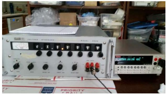
Change first decade dial to 6 for a reading of 6X0.0000. Adjust R904 for as close to 700.000000V as possible on the DMM.
