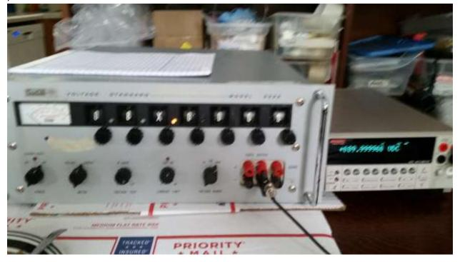
Change second decade dial to X for a reading of 0XX.0000. Adjust R912 for as close to 110.000000V as possible on the DMM.
