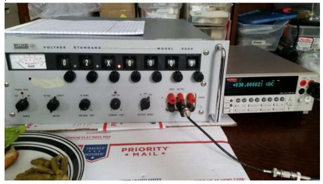
Change second decade dial to 4 for a reading of 04X.0000. Adjust R909 for as close to 50.0000000V as possible on the DMM.
