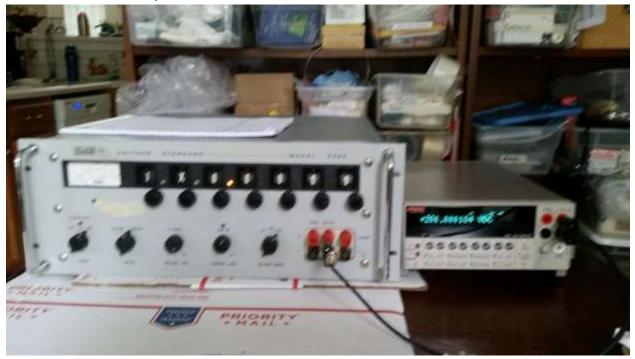
Change first decade dial to 2 for a reading of 2X0.0000. Adjust R902 for as close to 300.000000V as possible on the DMM.
