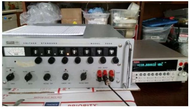
Change first decade dial to 1 and the third decade dial to 0 for a reading of 1X0.0000. Adjust R901 for as close to 200.000000V as possible on the DMM.
