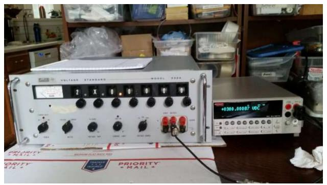
Change first decade dial to 4 for a reading of 4X0.0000. Adjust R903 for as close to 500.000000V as possible on the DMM.
