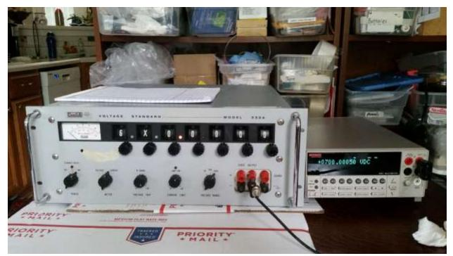
Change first decade dial to 8 for a reading of 8X0.0000. Adjust R905 for as close to 900.000000V as possible on the DMM.
