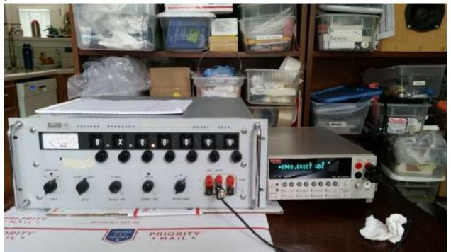
Change dials to read 1000.00000. adjust R906 for as close to 1000.0000V as possible on the DMM on the DMM.
