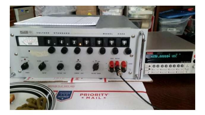
Change second decade dial to 6 for a reading of 06X.0000. Adjust R910 for as close to 70.0000000V as possible on the DMM.
