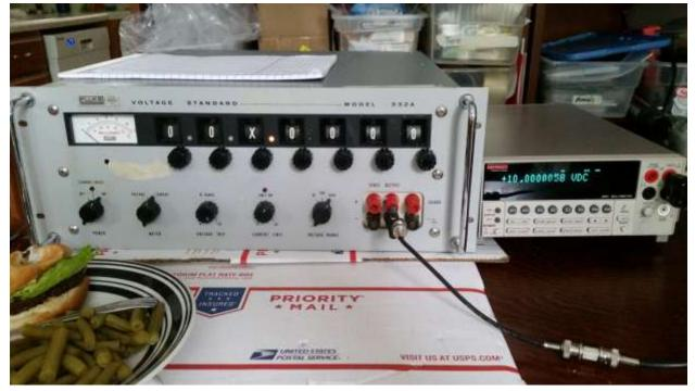
Change second decade dial to 1 for a reading of 01X.0000. Adjust R907 for as close to 20.0000000V as possible on the DMM.
