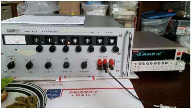
Change second decade dial to 2 for a reading of 02X.0000. Adjust R908 for as close to 30.0000000V as possible on the DMM.
