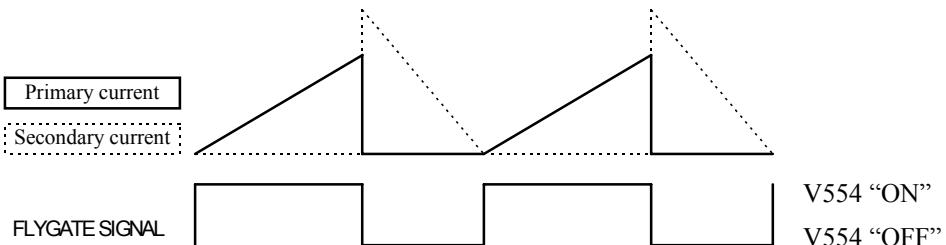
Figure 3-5. Fly-Back Converter Current and Control Voltage
