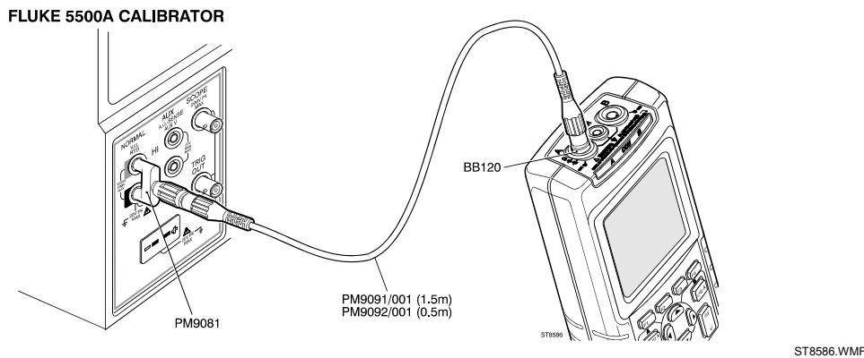
Figure 4-4. Test Tool Input 1 to 5500A Normal Output
