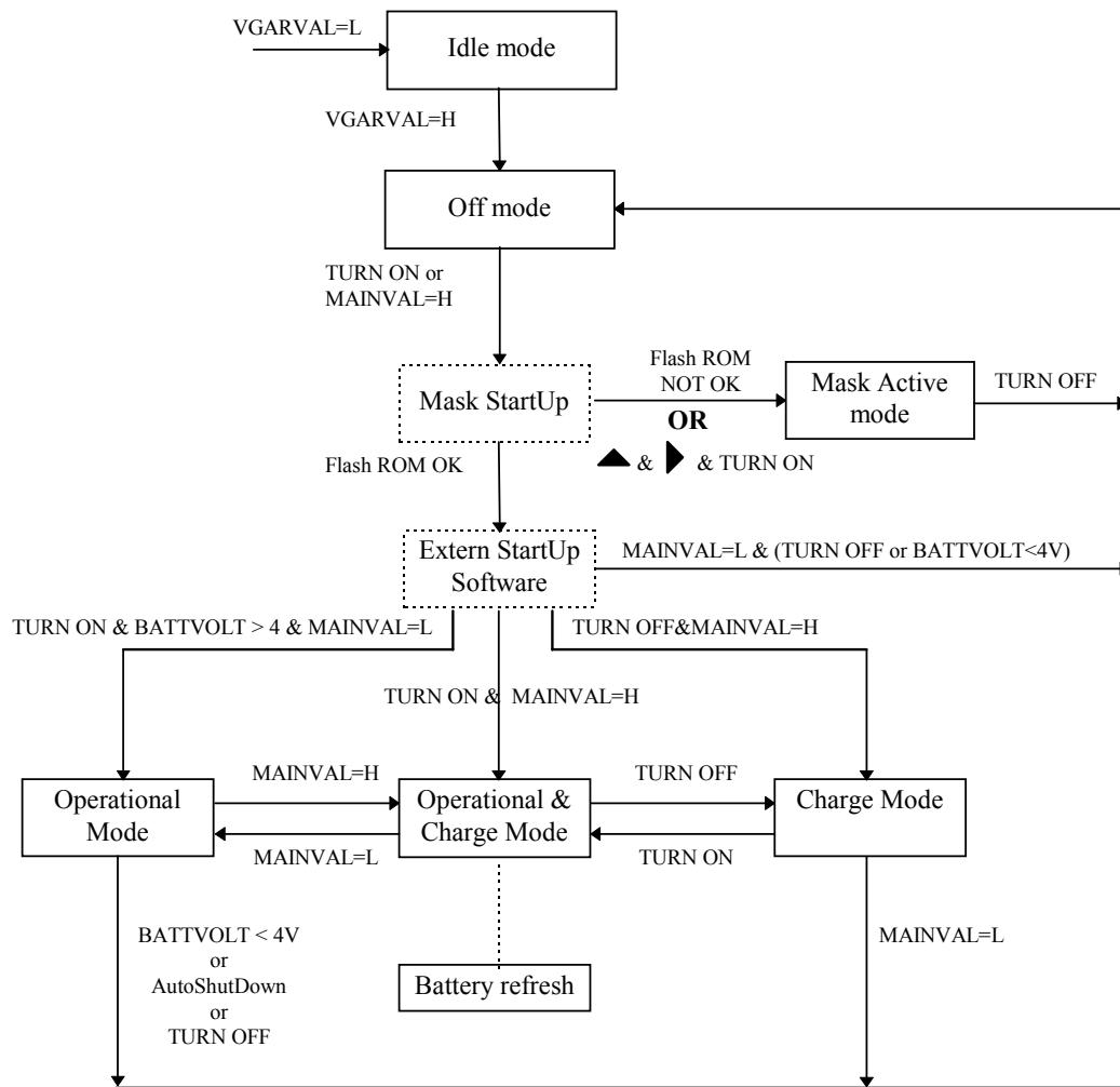
**Figure 3-2. Fluke 43B Start-up Sequence, Operating Modes**
