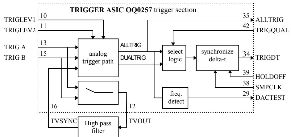
Figure 3-10. T-ASIC Trigger Section Block Diagram
