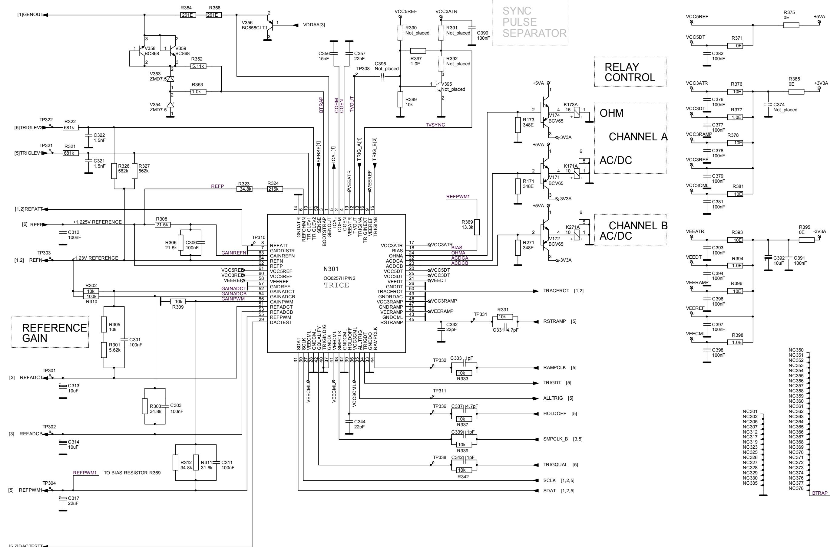
**Figure 9-4. Circuit Diagram 4, Trigger Circuit**
