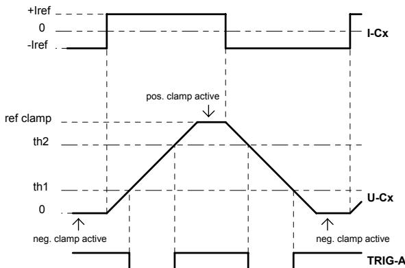
**Figure 3-9. Capacitance Measurement**
