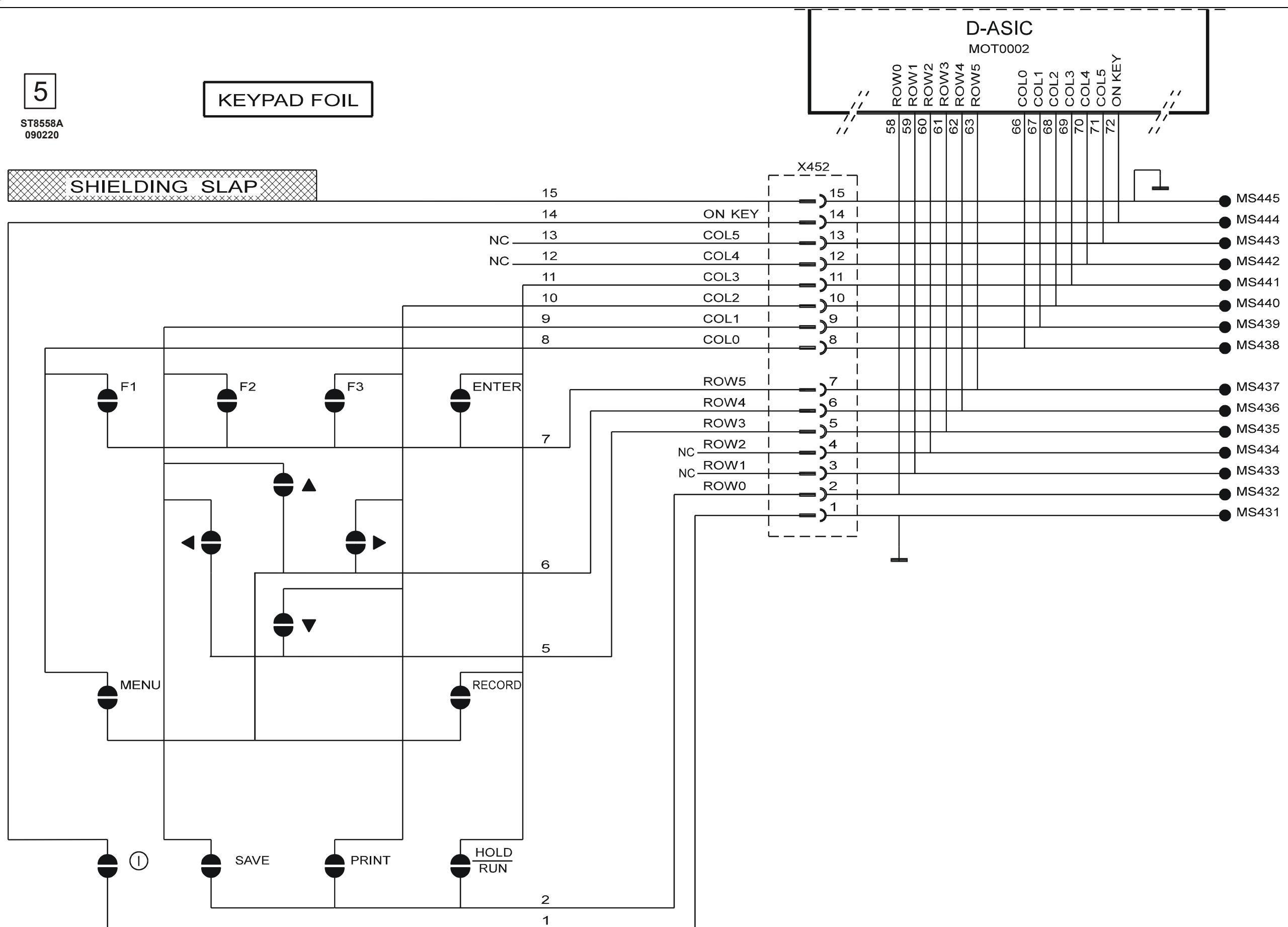
Figure 9-6. Circuit Diagram 5 (cont), Digital Circuit Keyboard
