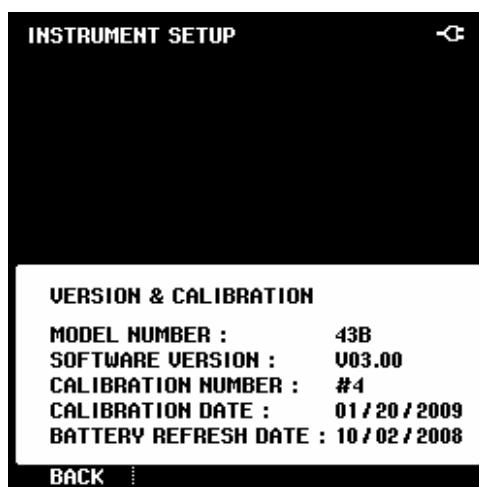
Figure 5-1. Version & Calibration Screen
