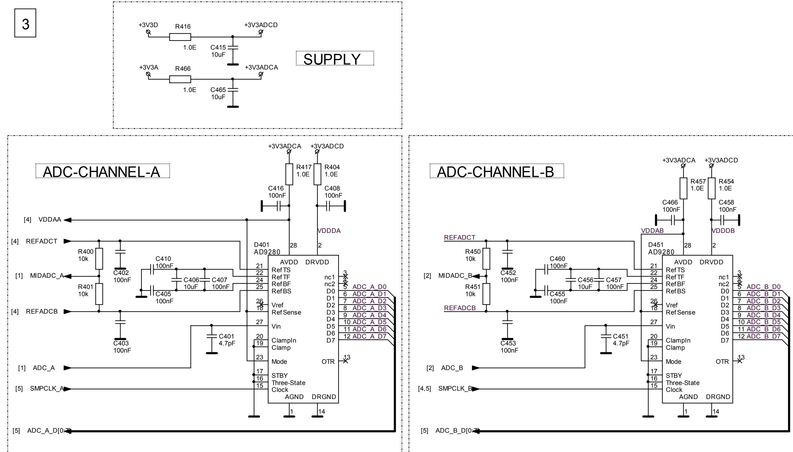
Figure 9-3. Circuit Diagram 3, Analog-to-Digital Conversion
