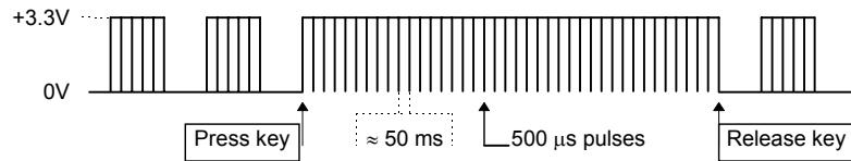
If no key is pressed the ROW lines are low if a battery is installed; if the Fluke 43B is powered by the the mains adapter only, the lines are alternating pulsing and low.
