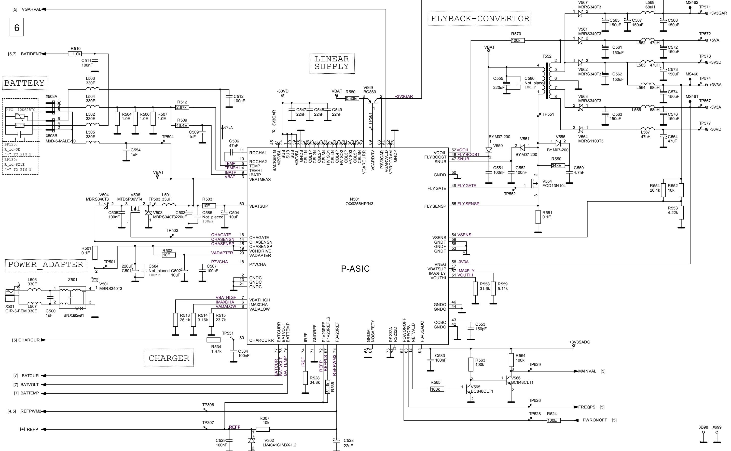
**Figure 9-7. Circuit Diagram 6, Power Circuit**
