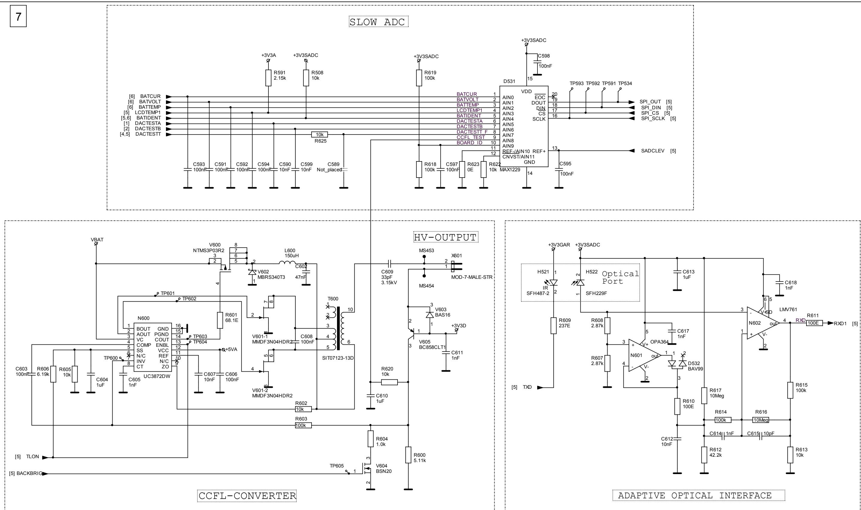
Figure 9-8. Circuit Diagram 7, Slow-ADC, Optical Interface, Backlight Converter
