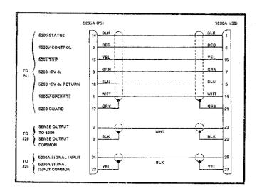
Figure 4-9. CALIBRATOR MODE INTERCONNECTIONS
