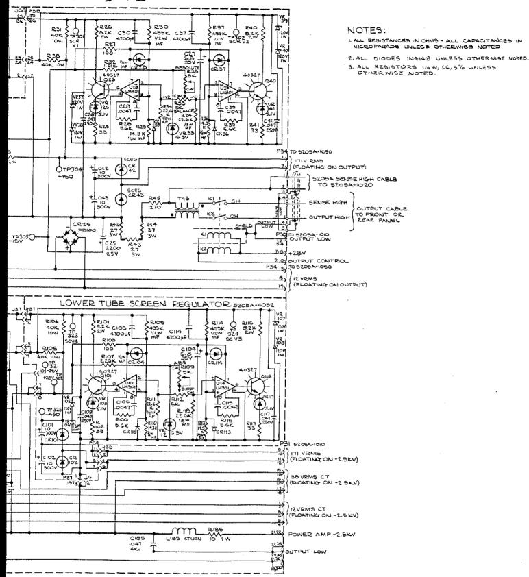
FIGURE 8-9. POWER AMPLIFIER ASSEMBLY (5205A-1030)
