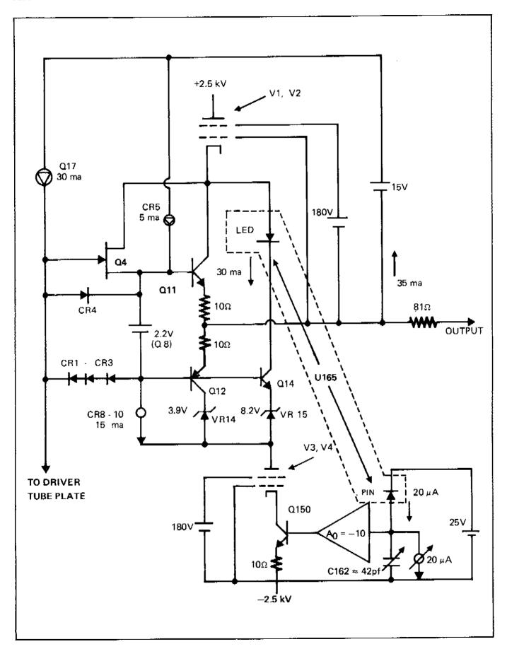
Figure 3-3. SIMPLIFIED POWER AMPLIFIER SCHEMATIC DIAGRAM
