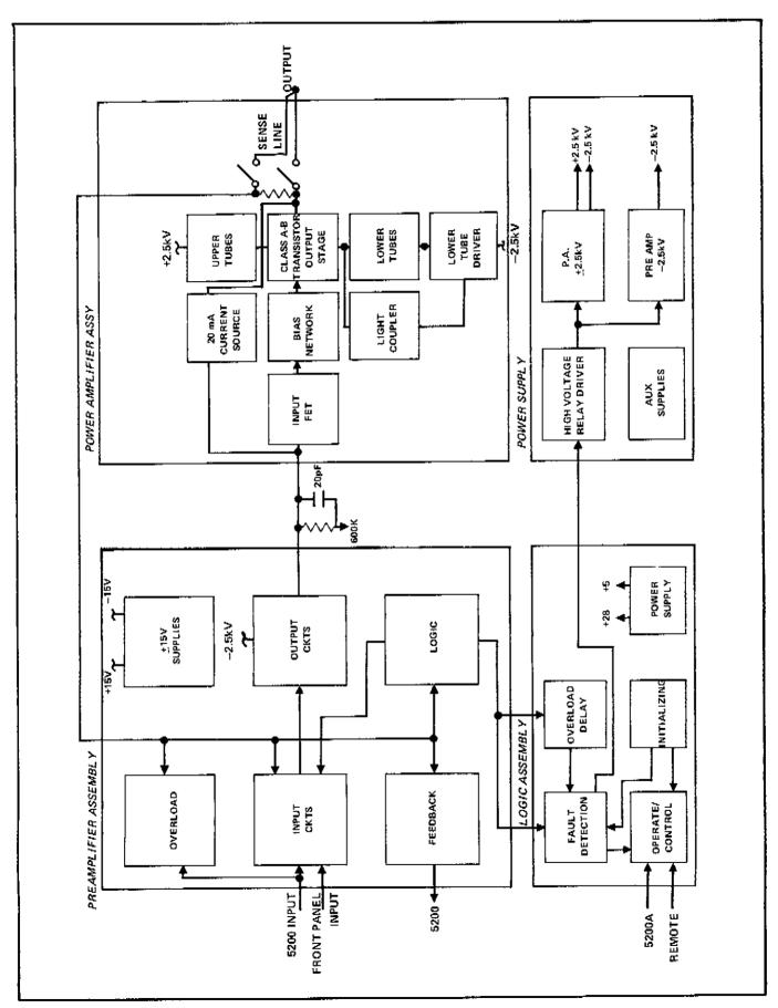
Figure 3-1. MODEL 5205A BLOCK DIAGRAM
