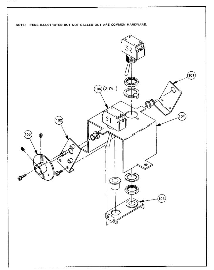
Figure 5-1. POWER SWITCHES VIEW
