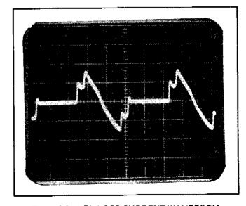
Figure 4-8. LED LOOP CURRENT WAVEFORM
