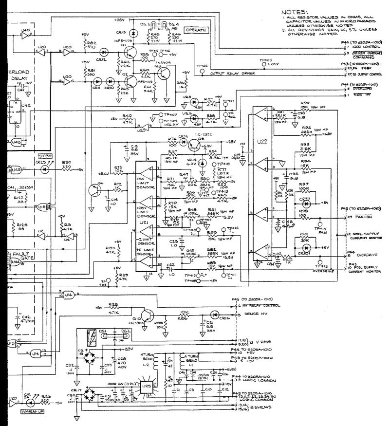
FIGURE 8-5. LOGIC PCB ASSEMBLY (5205A-1040)
