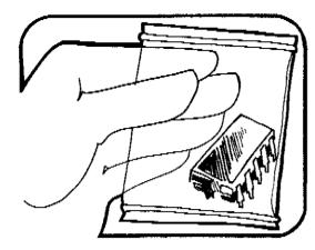
5. USE ANTI-STATIC CONTAINERS FOR HANDLING AND TRANSPORT
