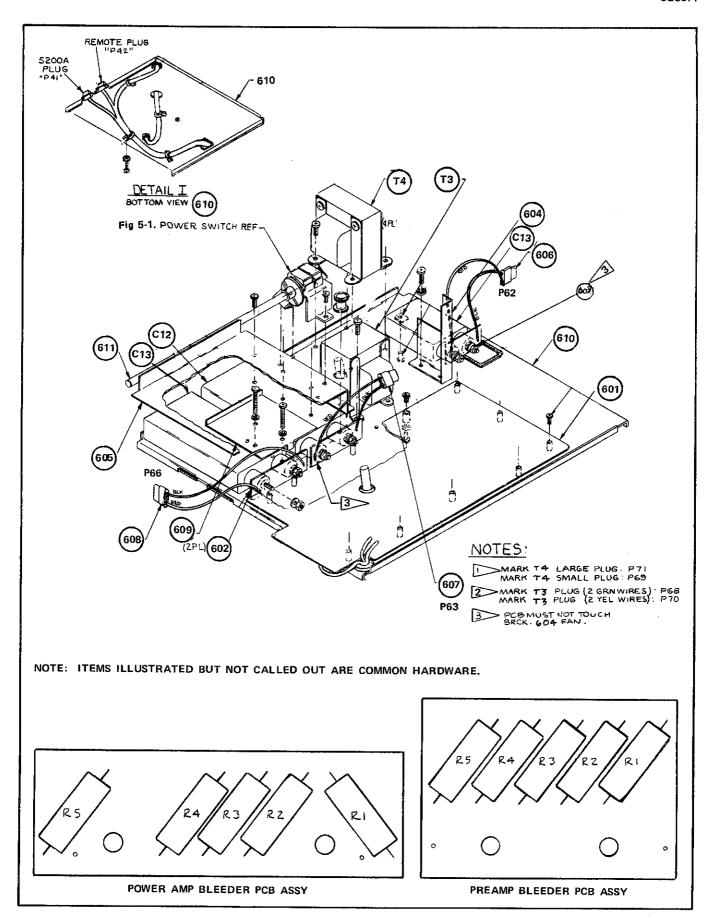
Figure 5-6. POWER SUPPLY VIEW
