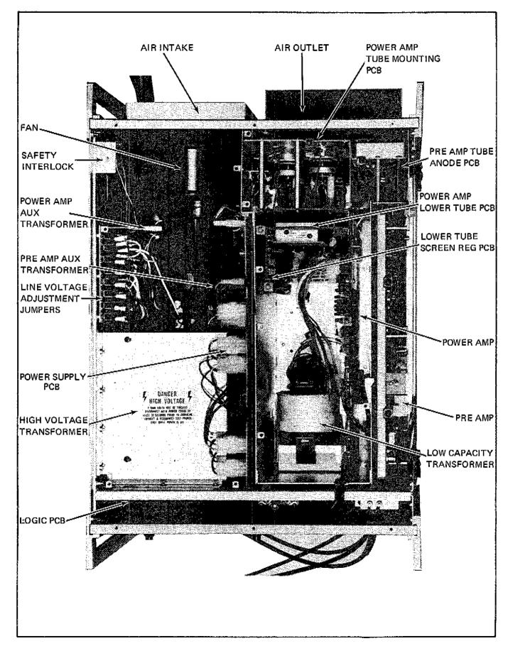
Figure 4-4, INTERNAL LAYOUT
