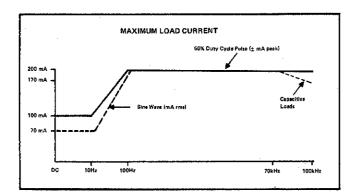
Bipolar Symmetrical wave form (See Graph above) Unipolar Rectangular waveform (Referenced to zero volts)
