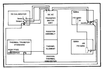
Figure 4-3. CALIBRATOR MODE CONNECTIONS
