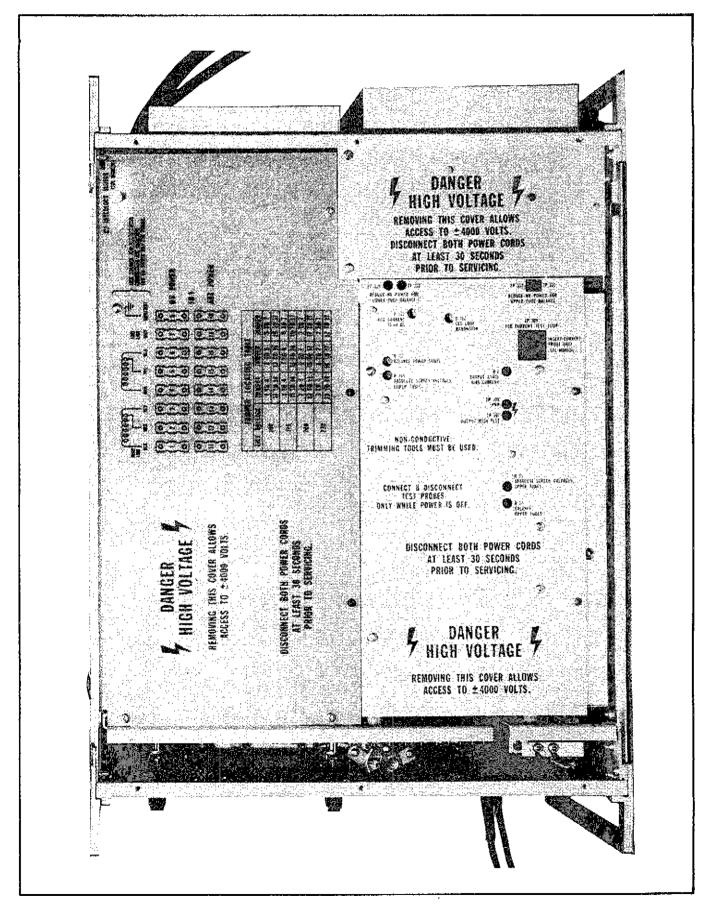
Figure 4-5. POWER AMPLIFIER ADJUSTMENT PORTS
