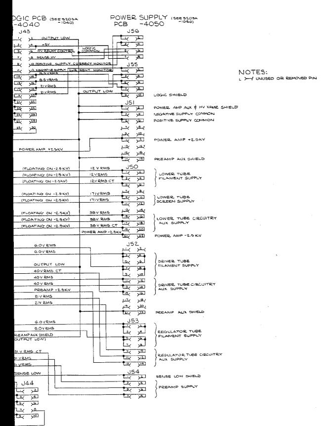
FIGURE 8-1. MOTHER PCB ASSEMBLY (5205A-1010)
