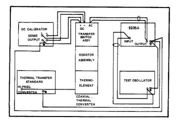
Figure 4-2. LOCAL AND REMOTE MODES CONNECTIONS.
