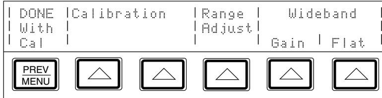
2. To calibrate the main output functions, press one of the softkeys under "Calibration." The display shows the following:
