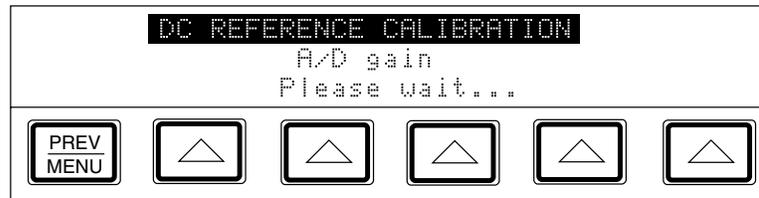
When the calibrator's 6.5V and 13V references have been characterized, the display shows the following message, which lets you accept or reject the changes that are about to be made to the calibration constants.
