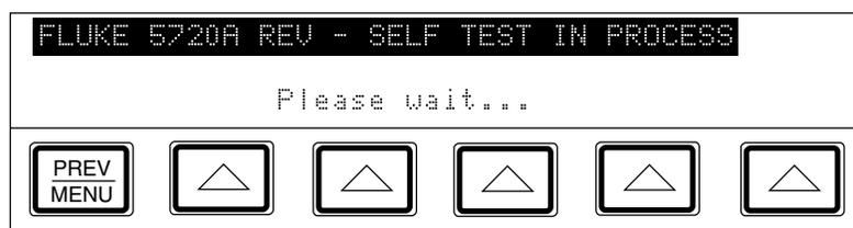
After the calibrator passes its self-tests, it powers up to 0V dc in standby, configured for internal sensing and internal guard, ready to accept an entry from the keypad. The Control Display now appears as shown below:
