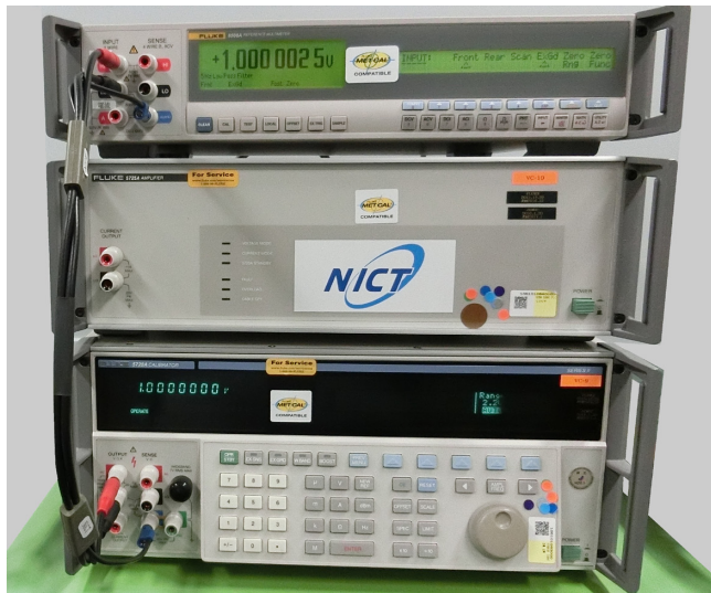
Fig. 2 Calibration of standard voltage and current generator (Top) Multi-meter: Fluke 8508A, (Middle) Amplifier: Fluke 5725A (Bottom) Standard voltage and current generator: Fluke 5720A
