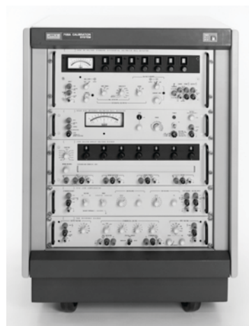
Fig. 1 Fluke 7105A calibration system
