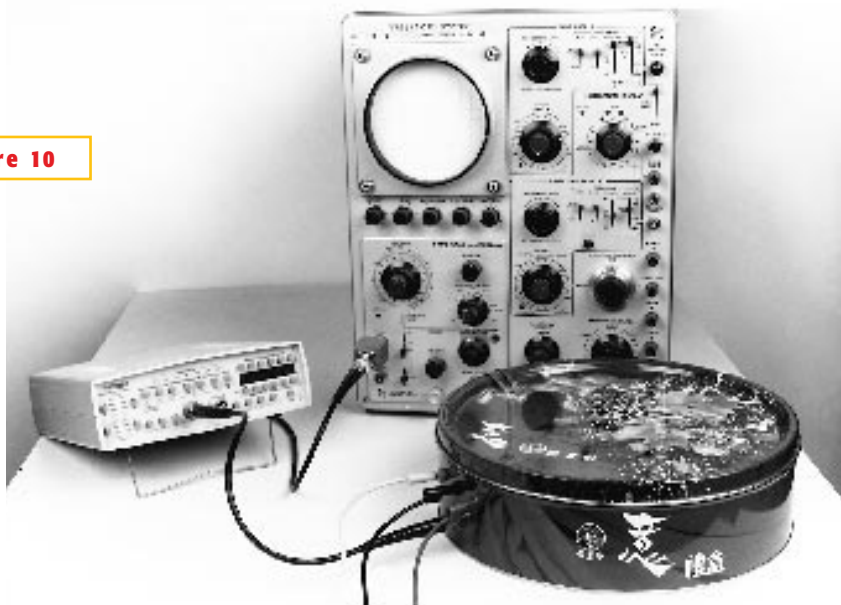
The noise-measurement test setup includes a shielded DAC breadboard (foreground), a preamplifier (left), and a lowpass filter attached to the oscilloscope (center). The measurement path is fully coaxial.
