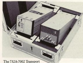
Case is a ruggedized, fiberglass, foam-lined case capable of holding a 732A dc Reference Standard and a 732A-7003 Battery Charger, complete with up to four 732A-7005 Battery Packs. This extra battery capacity plus the heat-conserving insulation of the foam-lined case will extend the off-line operating time of the 732A to about 72 hours.
