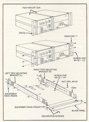
Installing the 732A-7004 rack tray kit.
