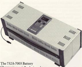
Charger is specially designed to hold and charge from one to four Battery Packs with the proper constant current, constant voltage cycle to avoid damage from over-charging. Fully discharged batteries are returned to approximately 95% charge in 24 hours. The charger provides the necessary isolation diodes and interconnections to provide the optimum charge to battery packs that may have unequal capacities or states of charge and connects the batteries to the 732A dc power input connector.
