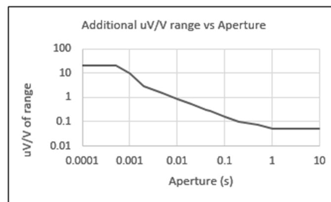
Aperture  $\geq 100 \mu\text{s}$ ; additional uncertainty with read rate: (Period = aperture + delay between readings)
