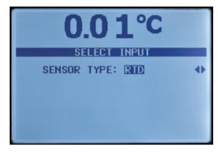
Use arrow keys to select mA (for transmitter), TC (for thermocouple) or RTD.
