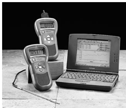
LogWare software can be used to graphically and statistically analyze data logged to the Model 1522 LLL. LogWare can also turn either Handheld Thermometer into a real-time datalogger.
