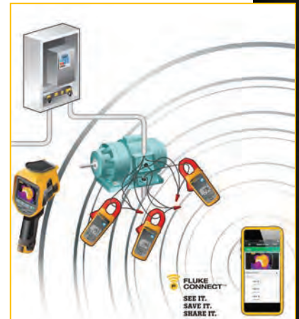
Measuring Three-phase load draw with Fluke Connect Wireless Tools
