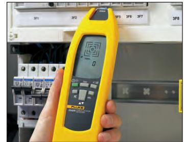
Location of fuses/breakers and assignment to circuits
