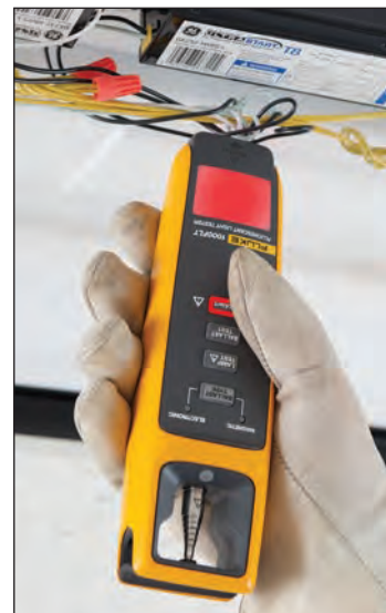
Non-contact voltage: Quickly check for voltage presence
