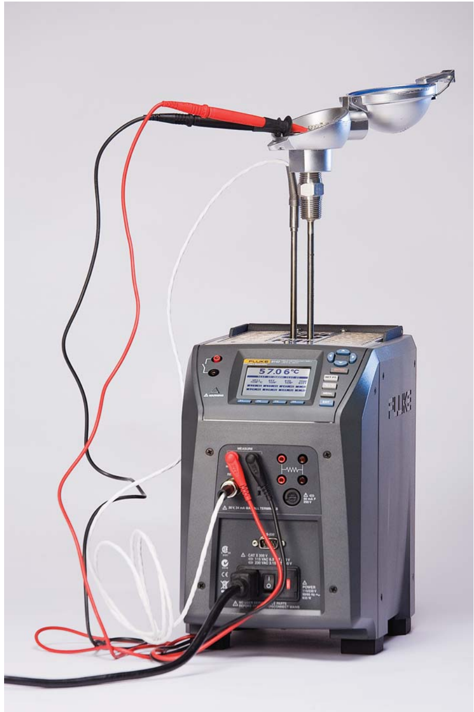
With the ability to measure a reference PRT, mA current, and source 24 V loop power, Field Metrology Wells can automate and save up to 20 different tests.
