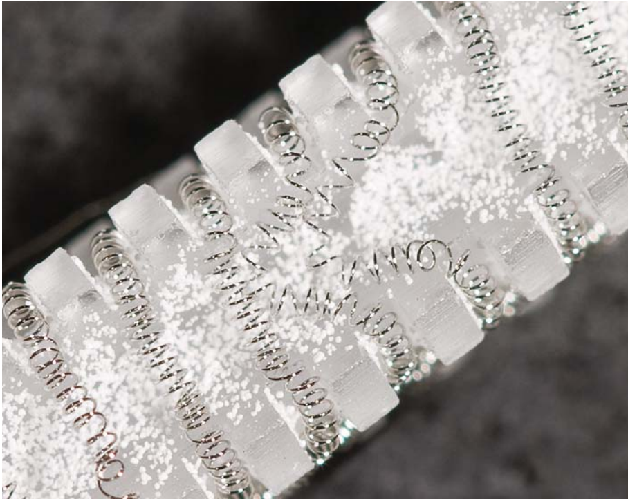
Damaged coils from a dropped sensor.
