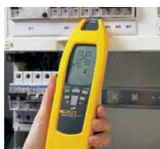
Location of fuses/breakers and assignment to circuits
