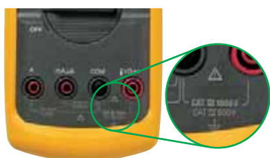
Use meters with these markings: 1000 V CAT III or 600 V CAT IV
