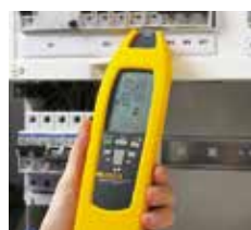
Location of fuses/breakers and assignment to circuits
