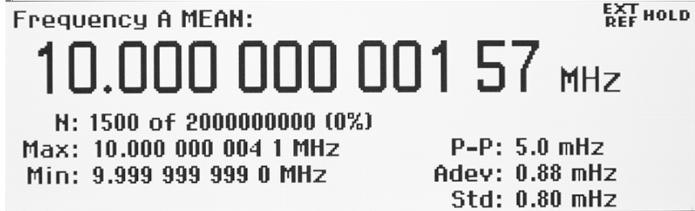
HP Z 3805A as extRef and DUT smart Freq off_1 Sec GateTime Stat.JPG (106.57 kB, 791x241 - viewed 106 times.)
