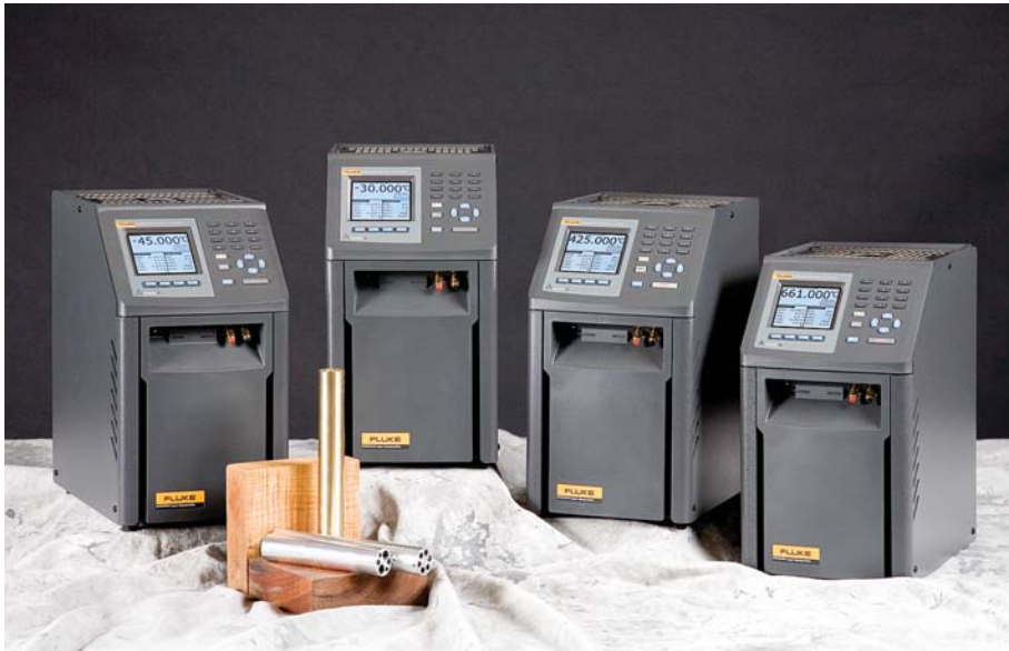
The Metrology Well family consist of four models (Model 9170, 9171, 9172, and 9173) which, combined, cover a temperature range of -45 °C to 700 °C.
