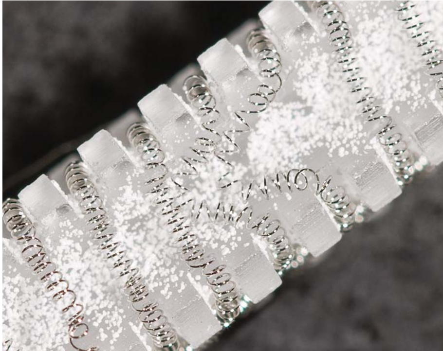
Damaged coils from a dropped sensor.
