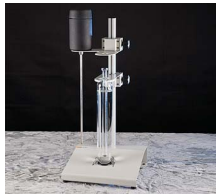
Hart's 2031A "Quick Stick" Immersion Freezer offers unmatched convenience and simplicity in forming the triple point of water ice mantle.
