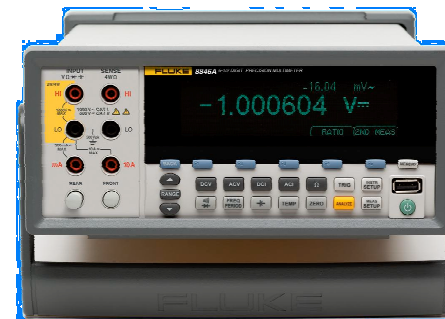
The UUT: Direct Voltage for a Fluke 8846A
