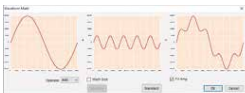
Sine+(1/4 Amplitude& 5 Times freq.) Sine Waveform
