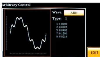
Clipped Sinewave Simulate Grid Power Supply Heavy Load Waveform
