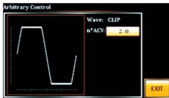
Clipped Sinewave Simulate Grid Power Supply Heavy Load Waveform
