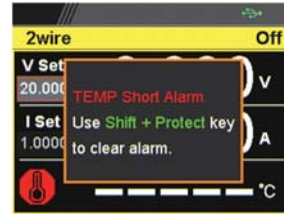
Red: The Alarm of Short Circuit Occurs From Temperature Measurement
