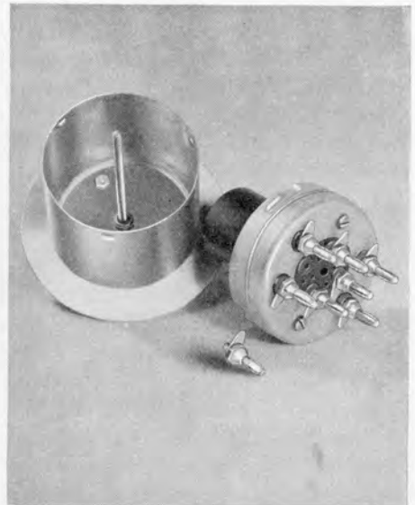
FIGURE 8. The shield base is securely locked to the shield top by the three bayonet catches to make a single unit. In the center is the threaded rod which engages a threaded insert in the jack base and draws the cover plate firmly against the panel. One plug has been removed to show small holes for lead wires
