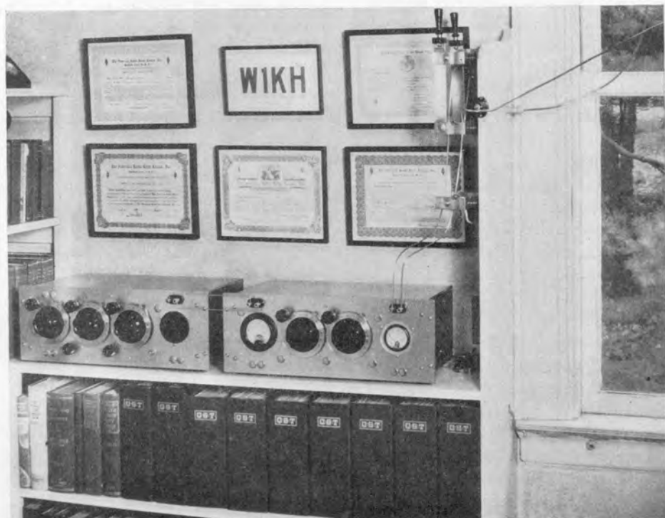
This transmitter was assembled from General Radio Unit Panels and Accessories. The exciter unit at the left duplicates the one shown in Figures 1 and 2. Photograph by courtesy of WIKH, Mr. George W. Bailey of Weston, Massachusetts
