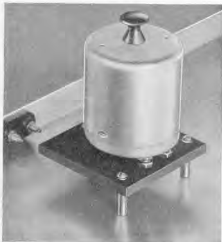
FIGURE 9. The jack base can, if desired, be mounted on a horizontal base plate to accommodate a shielded inductor as shown here. Note also that the unshielded inductor unit can be used in this jack base
