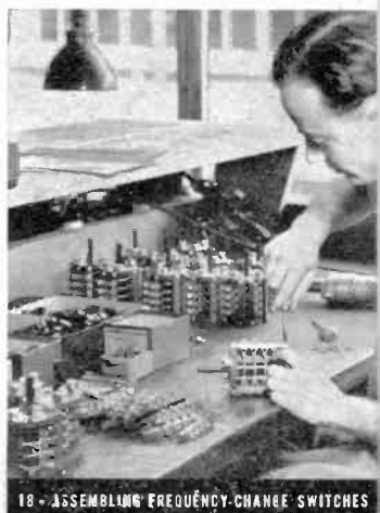
18 - ASSEMBLING FREQUENCY-CHANGE SWITCHES
