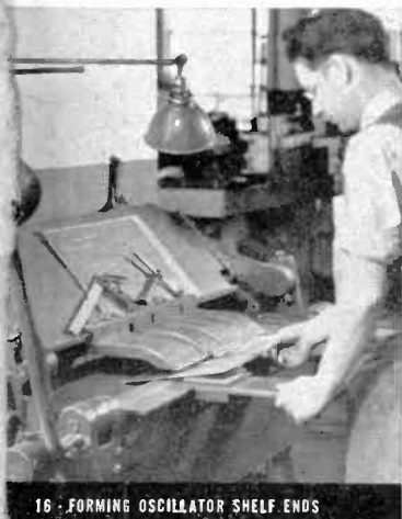
16 - FORMING OSCILLATOR SHELF ENDS
