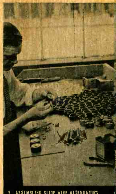
9 - ASSEMBLING SLIDE WIRE ATTENUATORS
