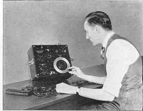
Testing condensers with the TYPE 740-B Capacitance Test Bridge.
