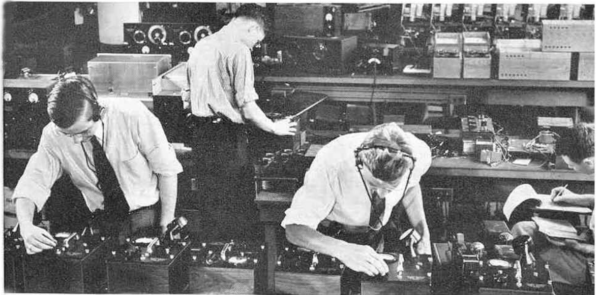
Above—Calibrating Type 724-A Precision Wavemeters in the standardization laboratory. Below—Analyzing fan noise with the Type 760-A Sound Analyzer.
