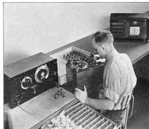
Measuring radio-receiver coils with the TYPE 721-A Coil Comparator.
