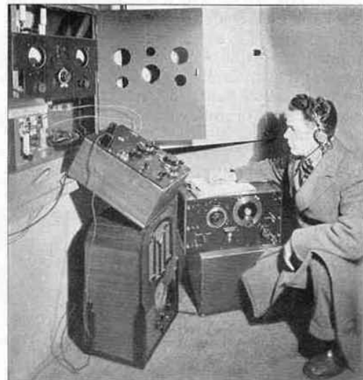
The photograph above shows the bridge with TYPE 684-A Modulated Oscillator set up for measuring antenna characteristics in a radio broadcasting station.
