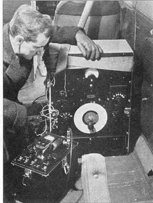
Testing the experimental model of TYPE 736-A Wave Analyzer under unusually severe operating conditions. This photograph was taken during an airplane flight to determine the frequency spectrum of airplane noise.
