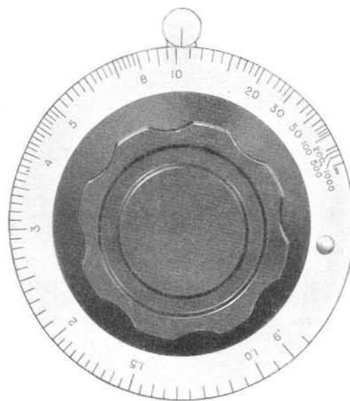
The MEGOHMS dial of TYPE 544-B Megohm Bridge. The scale is approximately logarithmic over the main decade from 1 to 10.
