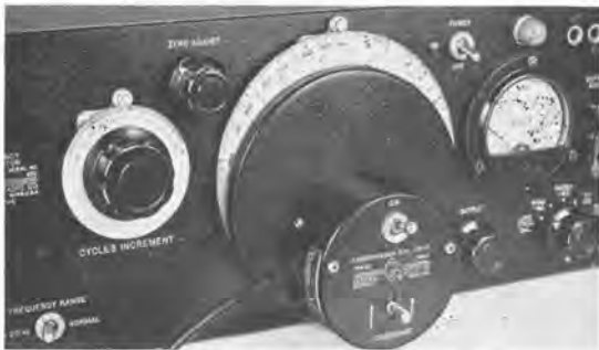
TYPE 908-P Dial Drive mounted to drive the frequency control of TYPE 1304-B Generator.
