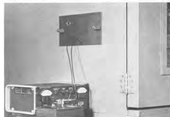
The built-in guard circuit permits the use of long leads from Comparator to sample inside conditioning chamber, as shown above.
