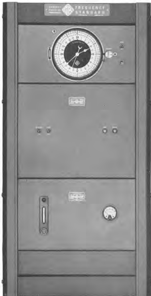
Close-up view of the TYPE 1100-AP Primary Frequency Standard. Lower part of the floor-type relay rack is not shown. The complete rack is similar to that shown in the photograph on page 77.
