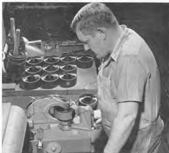
The coils for Variac® autotransformers are wound on the GR-designed machine, shown above, which applies an evenly spaced winding, accurately banked.
