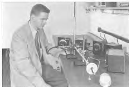
Admittance Meter set up with component mount and adjustable line to measure resistors at 500 megacycles.
