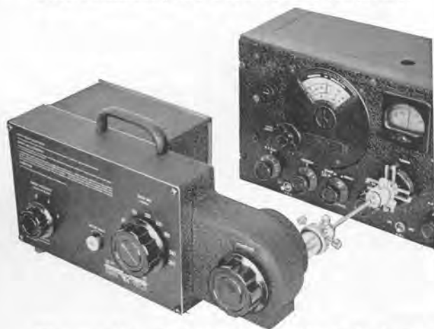
The sweep drive attached to the tuning knob of a short-wave receiver.
