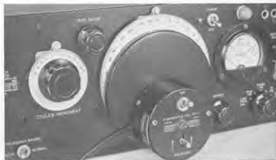
TYPE 908-P2 Synchronous Dial Drive mounted on a TYPE 1304 Beat-Frequency Audio Generator.
