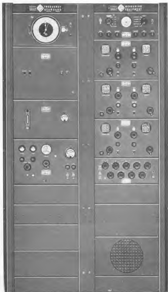
View of TYPE 1105-A Frequency Measuring Equipment with TYPE 1100-AP Primary Frequency Standard. The measuring equipment assembly is supplied with one floor-type relay rack, and the TYPE 1107-A Interpolation Oscillator mounts in the frequency standard rack, below the standard.
