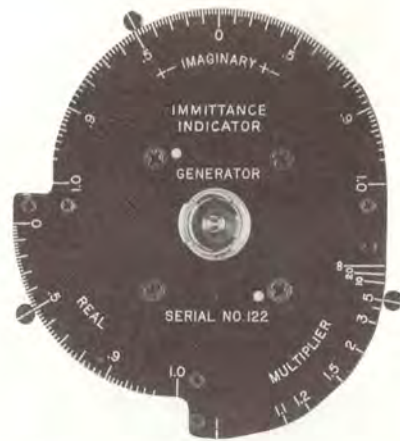
Dial calibrations of Transfer-Function Indicator (left) and Imittance Indicator (right).
