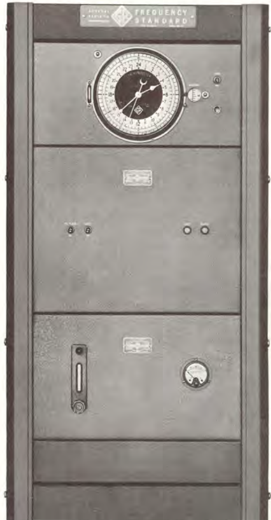
Close-up view of the TYPE 1100-APV Primary Frequency Standard. Lower part of the floor-type relay rack is not shown. The complete rack is similar to that shown in the photograph on page 76. The voltage regulator is not shown in either view.
