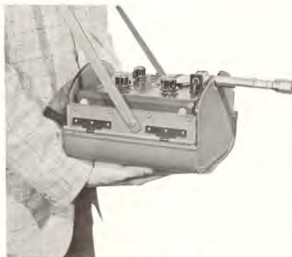
The Sound-Level Meter is being operated while in the leather carrying case and the microphone in the horizontal operating position.
