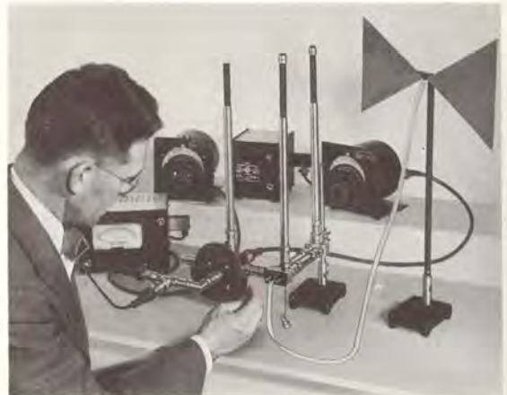
Figure 6. TYPE 874-Z Stands used to provide support for elements of a coaxial system.
