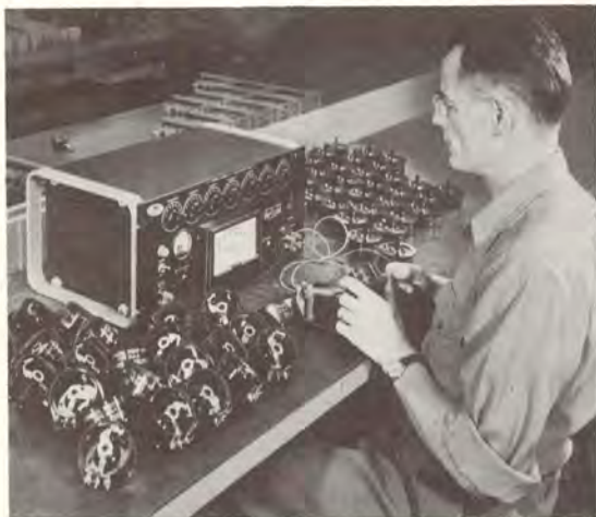
Resistance Limit Bridge used for production testing of potentiometers.
