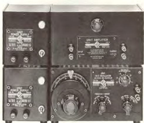
TYPE 1206-B Amplifier used with the TYPE 1210-C Oscillator.
