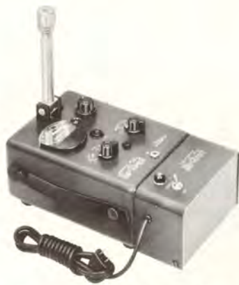
The TYPE 1551-B Sound-Level Meter ac operated from the TYPE 1262-B Power Supply and the microphone in the vertical operating position.
