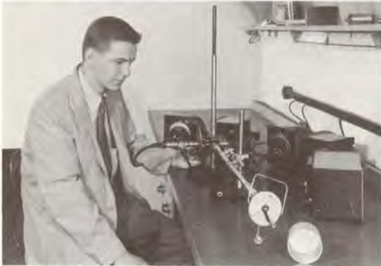
Admittance Meter set up with component mount and adjustable line to measure resistors at 500 megacycles.
