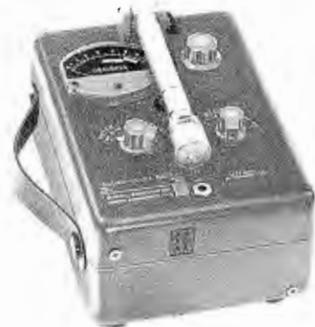
The Type 1551-C Sound-Level Meter with the microphone in the storage position and batteries automatically disconnected.
