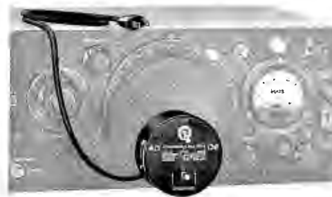
Motor drive attached to a Type 908 dial on the Type 1304-B Beat-Frequency Audio Generator.
