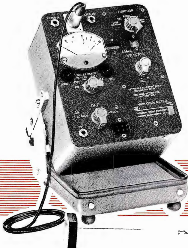
The Type 1553 Vibration Meter can be furnished with calibration in either English or metric units. The portable model in the convenient Flip-Tilt case is shown here. A rack-mount model is also available, as listed on the opposite page.
