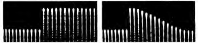
Expanded picture of line voltage peaks shows typical response of regulator. Left, 2% step change in input voltage; right, resulting output transient.
