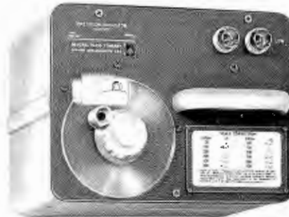
Two aluminum extrusions are strip-locked together to form the sides, heavy aluminum panel and bottom plate are added, and this precision capacitor is given the excellent shielding and trim appearance of the lab bench cabinet.
