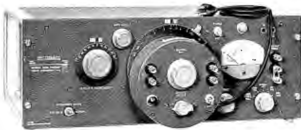
Type 1304-B Beat-Frequency Audio Generator driven by a Type 908-R96 Dial Drive, for use with an XY plotter.
