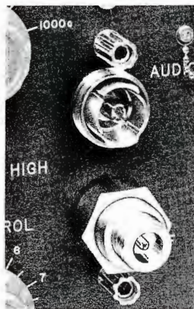
locking Type 874 panel connector adapted to type N with Type 874-QNJJ
