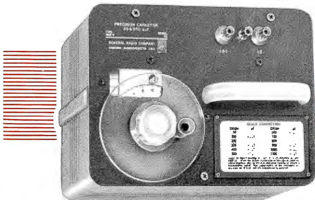
Panel and interior views of Type 1422-D Precision Capacitor.
