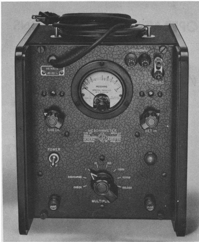
Panel View of the Type 1862-A Megohmmeter
