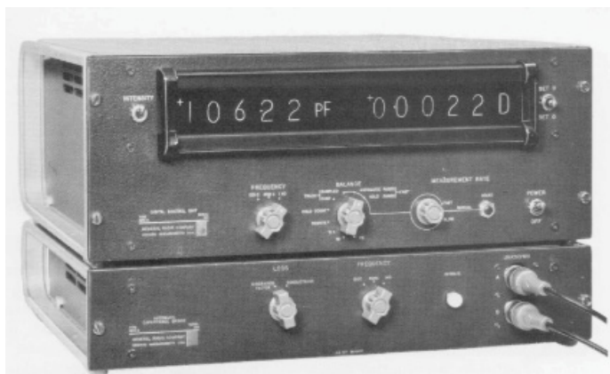
The 1680 Automatic Capacitance Bridge
