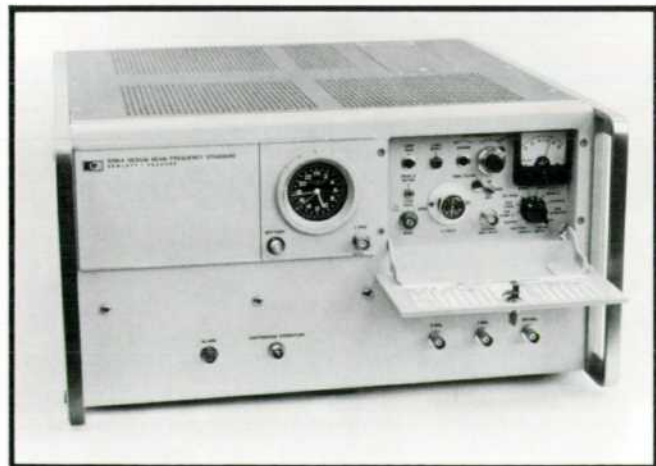
Fig. 1. HP 5061A Cesium Beam Frequency Standard is now available with standard or new high-performance cesium beam tubes. The high-performance tube's specifications guarantee 30% better accuracy, ten times better short-term stability, seven times better settability, and a factor of ten reduction in sensitivity to external dc magnetic fields.
