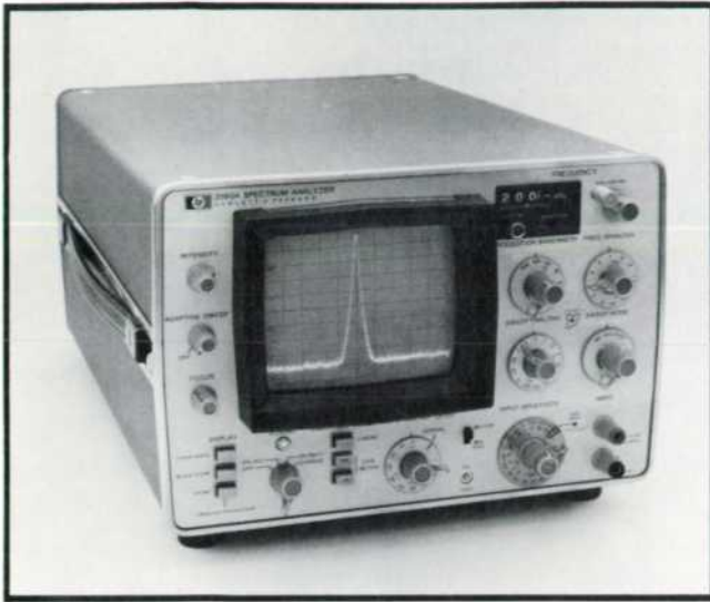
Fig. 1. Model 3580A Spectrum Analyzer spans a 5 Hz-50 kHz frequency range with frequency sweeps optimized for narrow-band selectivity. Even at very slow sweep rates, a flickerless display is obtained through use of digital storage.
