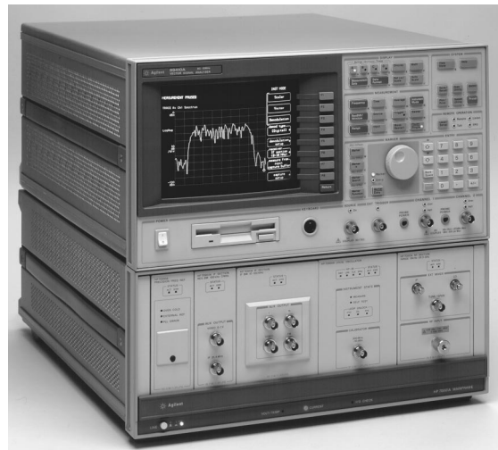
Figure 1. The Agilent 89410A vector signal analyzer and 71910A wideband surveillance receiver together form a wideband vector signal analyzer system.
