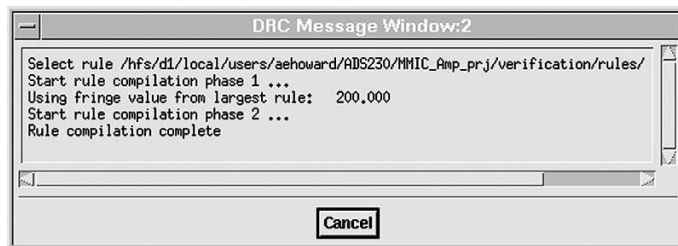
Figure B-2. Dialog box, showing that the rules file has been compiled.
