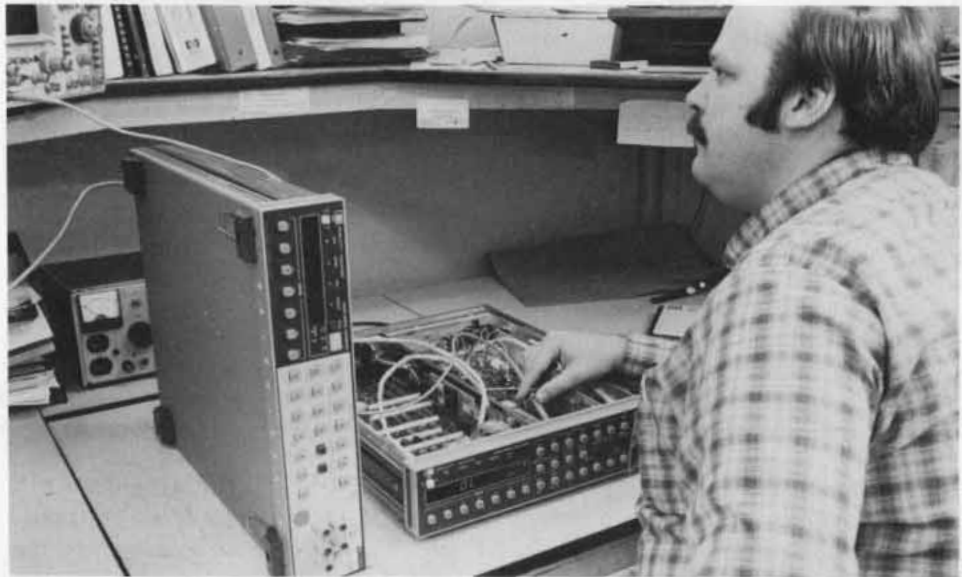
Figure 1. Mike Keenan, HP Technical Specialist, substitutes part of a good DVM into a faulty unit as a form of half-splitting.
